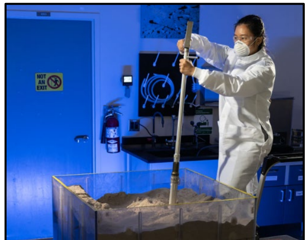
Image 1: Tools Engineer Yisha Ng hammers a Drive Tube into a densified lunar simulant testing bin, collecting a core sample of simulant material. (tools used: Hammer, Extension Handle, Drive Tube from government reference design tool kit).
