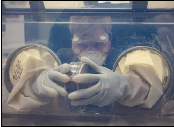
Image 2: Test Engineer James O'Hara examines an astronaut glove wrist connector seal in a dusty lunar simulant environment in a glovebox in the SDL.
